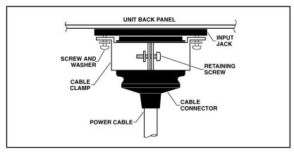
Figure 4.2: Input Cable Clamp Installation
